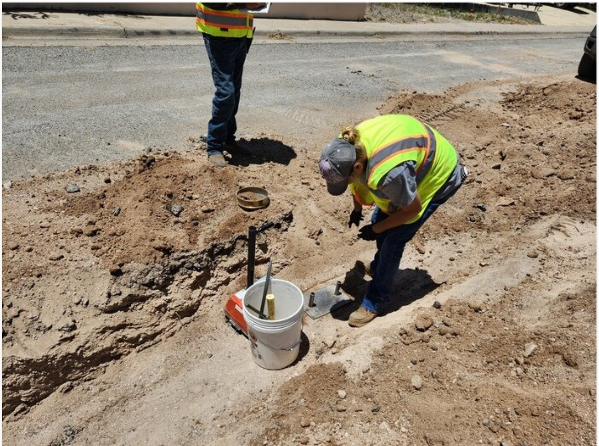
Summit testing technician taking densities on 12" C-900.
